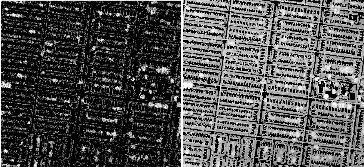
Figure 2.8: Image layer 'ElevationMax' before (left) and after filling of gaps in 2 cycles (right)
