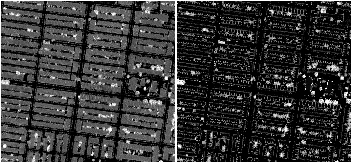
Figure 2.5: Layer 'NumberOfPoints' that represents the number of points in the point cloud that are mapped to a pixel (left) and 'ElevationStdDev' based on point property standard deviation of elevation (right).
