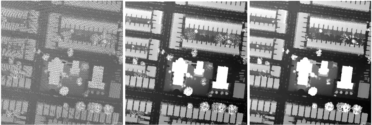
Figure 1.4: Rasterized DTM (left) with gaps filled (middle) and median filter applied (right) to remove outliers.
