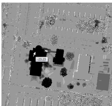
Figure 3.4: Elevation difference layer ' ElevationMax_after ' - ' ElevationMax_before ' - resulting in negative values for disappeared features
